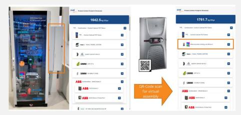
Left shows the control cabinet and its digital twin without the climate control unit (orange box). The blue box of the digital twin shows the current PCF value. When the climate control unit is added in the assembly process, the ID-Link can be scanned to retrieve the product information for the climate control unit. This information can than automatically be used to update the digital twin of the now completely assembled control cabinet, including its PCF value.
