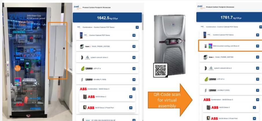
Left shows the control cabinet and its digital twin without the climate control unit (orange box). The blue box of the digital twin shows the current PCF value. When the climate control unit is added in the assembly process, the ID-Link can be scanned to retrieve the product information for the climate control unit. This information can then automatically be used to update the digital twin of the now completely assembled control cabinet, including its PCF value.
